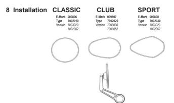
After aligning the mirror, the M5 clamping screw inside the arm is tightened with a torque of 4 Nm.
